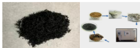
Figure 4. Schematic diagram showing biochar production in a slow pyrolyzer.
