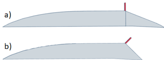
Figure 14. STL images of airfoils with propulsor “cell zones” in red, where: a) 25° taper, 10.55 cm height, 100.1 cm chord, and 5 cm X 0.5 cm propulsor and b) 45° taper, 10.4 cm height, 85.9 cm chord, and 5 cm X 0.5 cm propulsor at a -45° pitch.
