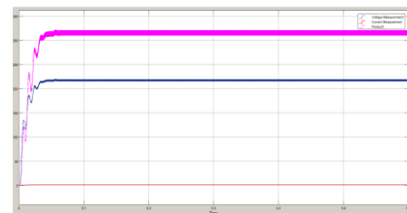
Figure 8. Voltage, output current, and power of a DC-DC converter with partial shading using P&O method
